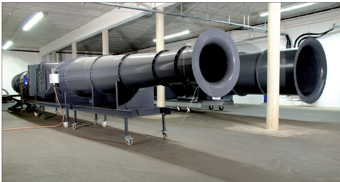
Suction side duct test rigs to determine the aerodynamic fan performance curve acc. ISO 5801 for axial fans of different diameters
